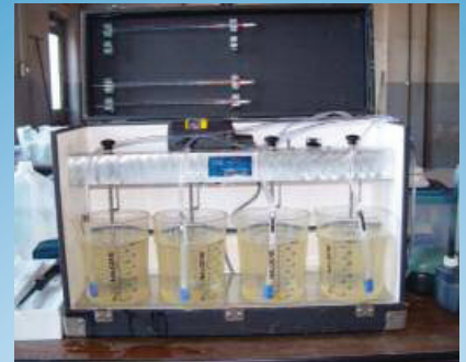
Modified Jar testing for testing ground waters with high iron
